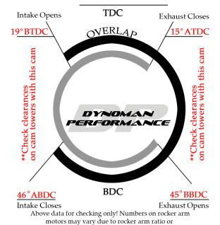
multiple valve jobs. Check at .050" Lift Off Seat with Valves Set At Running Lash
